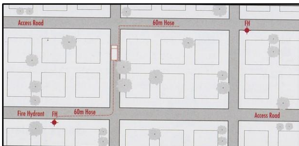
Figure 19 – Reticulated Fire Hydrant Coverage
