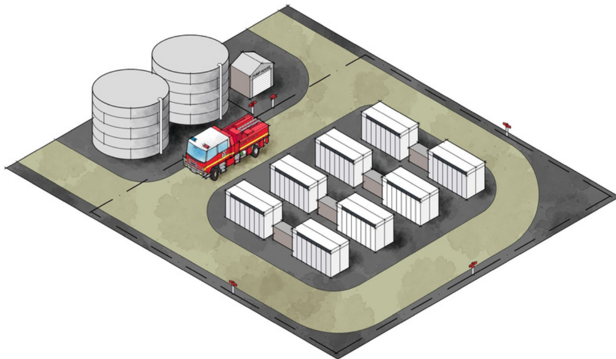
Figure 6: Best-practice arrangement of fire service infrastructure at facilities with battery energy storage systems without reticulated water supply, or a reticulated water supply that does not meet the performance requirements of AS 2419.1-2005: Fire hydrant installations.
