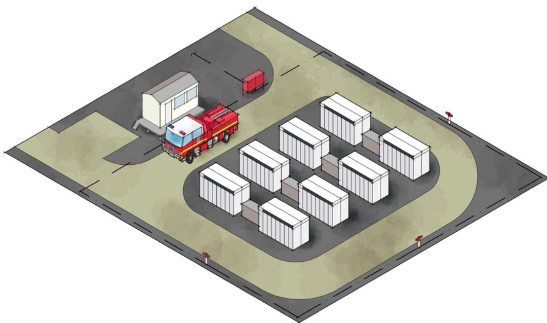
Figure 5: Best-practice arrangement of fire service infrastructure for facilities with battery energy storage systems with reticulated water supply meeting the performance requirements of AS 2419.1-2005: Fire hydrant installations .
