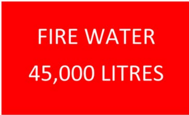
Figure 3: Fire water signage to comply with AS 2419.1-2005, Section 5.4.5: Fire hydrant tank signs.
