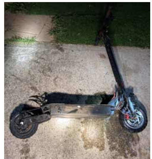
Clockwise from top left: Fire in bedroom caused by overloaded electrical equipment including lithium ion batteries. Fire in kitchen caused by defective scooter battery.
